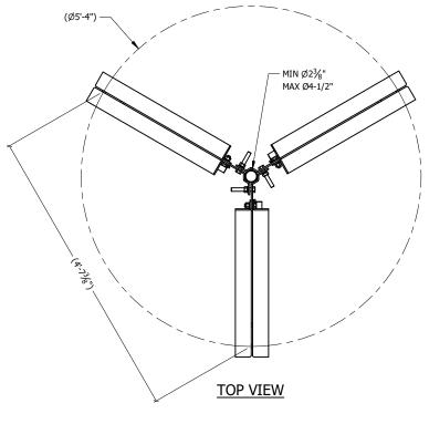
NOTES: \*THIS KIT CAN BE MOUNTED TO A NON-PENETRATING SLED. PART# RT4007 SOLD SEPARATE. \*THIS KIT CAN BE MOUNTED WITH CUSTOM PENETRATING
